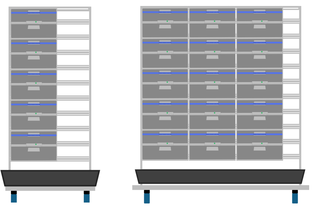
Triple TwinBin - 0.75m Rack 5 Per side / 1.5m Rack 15 Per side
